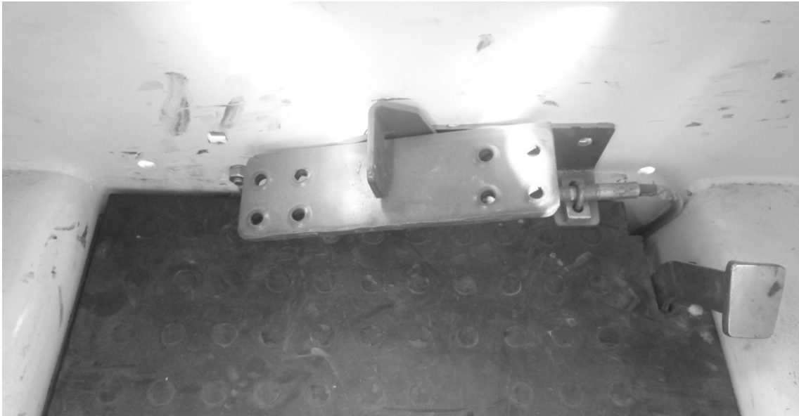
Figure 20 AUXILIARY HYDRAULIC CONTROL FOR THE ATTACHMENTS AND FOOT THROTTLE DEVICE
