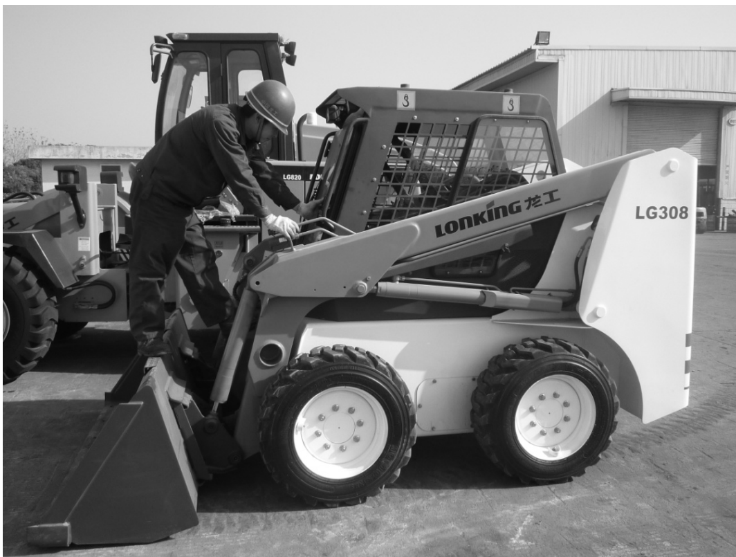
Figure 12 CORRECT WAY FOR MOUNTING THE MACHINE
