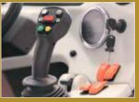
Electronic display with warning lights Joystick 5 and 11 functions. Maximum speed : indicating faults, engine, hydraulic 11-functions Joystick is standard on 12 Kmh LX models.
