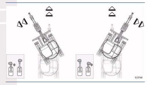
With the vehicle travelling straight AHEAD, both control levers will be pushed forward equally.
