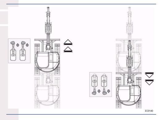
To begin FORWARD travel, move both control levers forward equally. As additional pressure is applied on the control levers, the machine's speed will increase. To STOP forward travel, slowly return both controls to their NEUTRAL (N) position.
