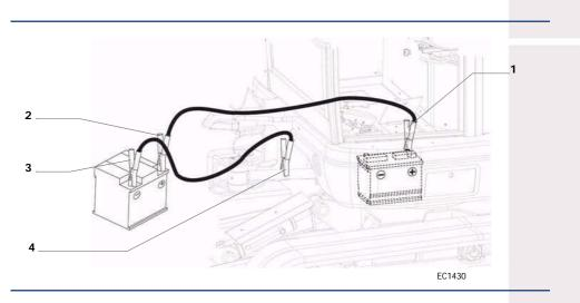
**1** - Connect one end of the positive (+) jumper cable to the positive (+) terminal of the flat battery (**1**) in the vehicle.
