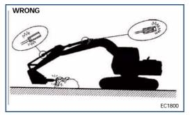
Stop work immediately if the hydraulic hoses bend in the wrong way. Then contact the dealer.
