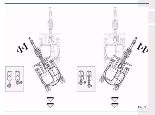
With the vehicle moving straight in REVERSE, both control levers will be pulled to the rear equally.
