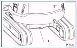
6 - When towing, keep the towing chain or cable taut throughout the operation.
