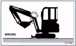
Do not engage the hydraulic hammer with the driving boom in a vertical position; excessive vibration on the driving cylinder may cause oil leaks.
