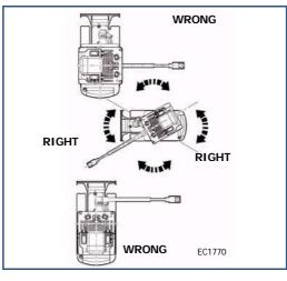
When operating the excavator, do not bump against the lifting boom with the hydraulic hammer.
