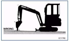
Do not run the hydraulic hammer for more than one minute at a time, since this may result in wear to the cutting edge or the hydraulics.
