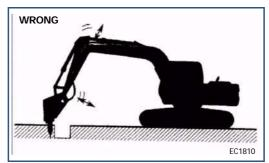
Do not operate with the hydraulic hammer in a sideways position; the machine will become unstable and the undercarriage components will be subjected to increased wear and tear.
