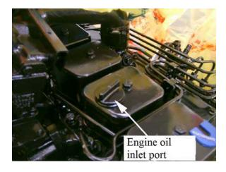
• Lay back the dipstick, close the side door on the cover of engine. For choosing the appropriate oil please refer to **CHAPTER IV 2.2 Oil Selection**.
