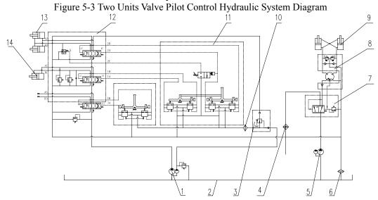
1-Work and Pilot Pump 2- Oil Tank 3- Pressure Select Valve 4-Hydraulic Oil Radiator 5- Steering and speed changing pump 6-Oil returning filter 7-Priority valve 8-Redirector 9- Steering Cylinder 10-Pilot Filter 11-Pilot Valve 12-Multi-way Valve 13-Lift-arm Cylinder 14-Bucket Cylinder
