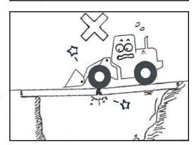
Make sure that every bridge is strong enough to let the machine pass.  Don't use the machine for any work other than what the machine is designed for. It may damage the parts or cause an accident when using the head of the working equipment for other fuctions, such as hook, grasp, draw, push, or tow.
