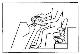
• Never lift the bucket to the highest position while transporting material. The lower hinge of the arm working equipment should be  $400\sim500$ mm above the ground to ensure stable driving in the transporting process.
