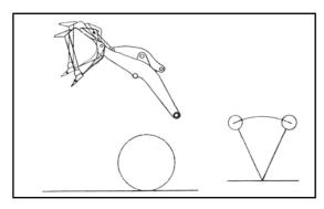
and gently during dumping to prevent the bucket from striking the ground.
