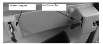
cab door will open. Turn the lock bar upward and it will open.
