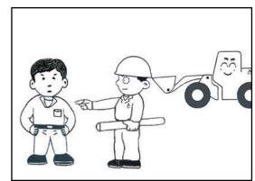
• Don't start the machine if there is the tag of "**NO OPERATION**" on the control handle of the working equipment or shift control handle.
