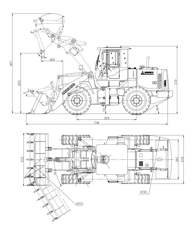
Figure 2-2 Geometrical dimensions of LG936L wheel loader mounted with standard lift arms
