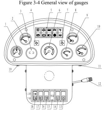
Gearbox Oil Pressure Gauge 2. Air Pressure Gauge 3. Working Chronometer 4. Left Turn Indicator Lamp 5. Indicator Lamp 6. Revolution Indicator 7. Right Turn Indicator Lamp 8. Fuel Level Gauge 9. Engine Water Temperature Gauge 10. Torque Converter Oil Temperature Gauge 11. Starting Switch 12. Switch Group 13. Water Spraying Switch 14. Rain Wiper Switch 15. Cover Board 16. Rear Lighting Lamp Switch 17. Front Lighting Lamp Switch 18. Rear Headlight Switch 19. Warning Lamp Switch
