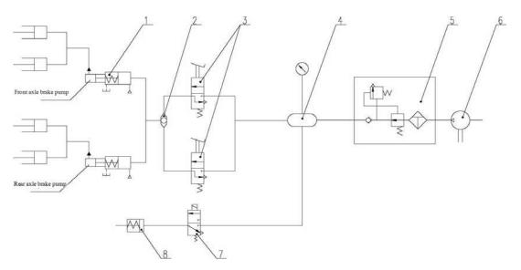
1- Air Booster Pump 2-Shuttle Valve 3- Air Brake Valve 4- Air Tank
