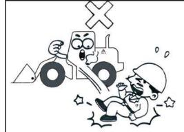
When getting on or off the machine, face the machine and use the handrails and pedals to ensure that you can support yourself. Keep at least three-point contact (two hands/one foot or two feet/one hand) with the handrails and pedals to ensure body stability.
