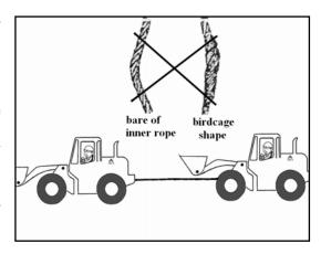
• Keep the hook of the towing machine and the towing parts in a horizontal line.
