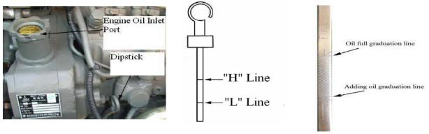
◆ Dongfeng Cummins 6BT5.9 engine: If the oil level is lower than the adding oil graduation line, oil should be added by the oil adding port. If it is higher than the oil full graduation line (FULL), check the problem and solve it. It is a suitable oil level if it is between the adding oil graduation line and the oil full graduation line (FULL).
