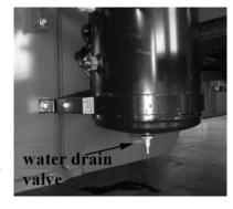
• Examine the outside of the air storage tank frequently because of high pressure air. Examine the anti- erosion layer and welding line to ensure safety.
