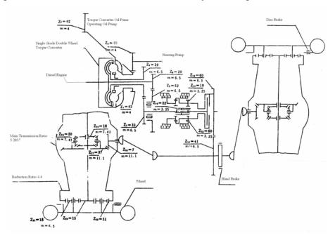
Figure 5-1 Principle Diagram of Transmission System
