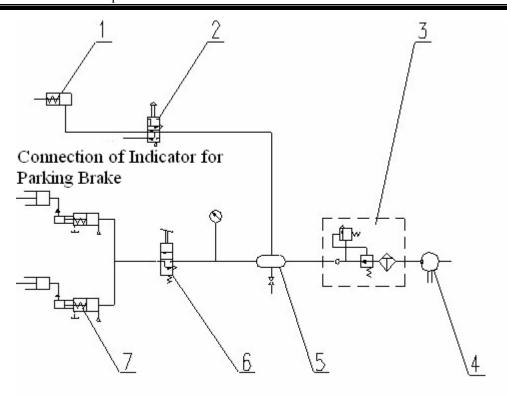
1-Parking Brake Air Chamber 2- Brake Magnetic Valve
