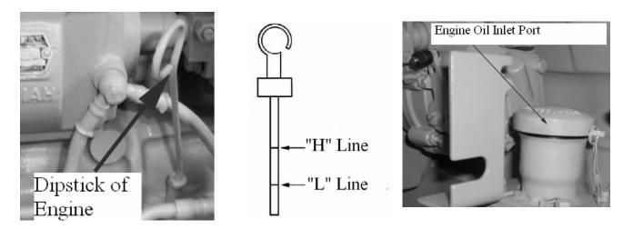
◆ Weichai TD226B engine: If the oil level is lower than the "L" line, oil should be added by the oil adding port; It is a suitable oil level if it is between the "L" and the "H" line.
