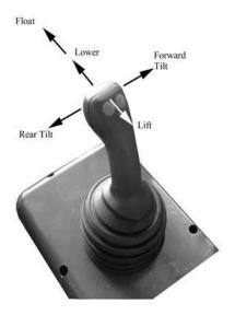
handle left to the rear tilt position and the control handle is locked. During drawing the bucket, the control handle returns to the neutral position and place it in the lowering position when in the set level automatically position. Then the equipment is placed on the ground and the bucket is in the bucketing position in order to realize the set level automatically function and increase the efficient of the whole vehicle.
