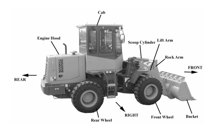
Figure 2-1 General view and components' name of LG936L wheel loader
