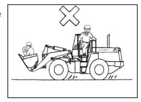
• Follow the traffic rules on the common roads. Pass the crossing road quickly and do not block the road.
