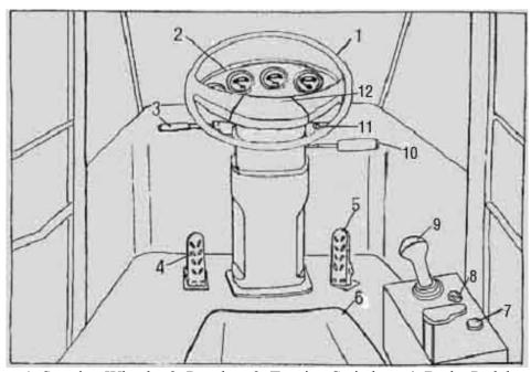
1. Steering Wheel 2. Panel 3. Turning Switch 4. Brake Pedal 5. Accelerator Pedal 6.Seat 7. Parking Brake Control Switch 8. Flameout Control Soft Knot 9. Equipment Control Lever 10. High and Low Speed Control Lever 11. Starting Switch 12. Horn Button
