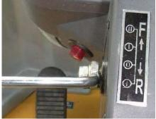
gear. Put the control lever forward to the 1 position can obtain the forward gear I, and the machine goes forward at low speed. When turn it to 2 position, the forward gear II can be obtained, and the machine goes forward at high speed. Putting the lever to R position can obtain the reverse gear and the machine goes backward.
