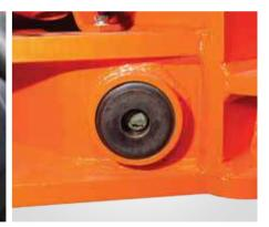
A new model of shock pad is used to provide stronger durability and reduced shock and noise, effectively relieving the driver's fatigue.
