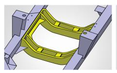
Connecting parts of swing frame adopt a reinforcement design to offer greater strength.
