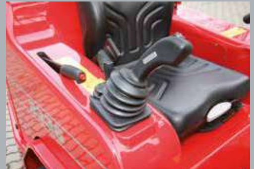
The slightly twisted joystick position simplifies operation.
