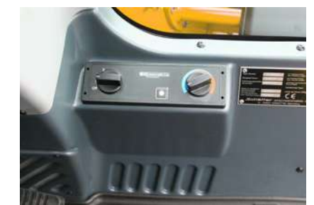
Heating with powerful, 3-speed blower
