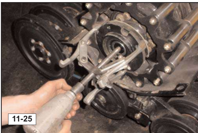
8. Use a jaw style puller and an impact wrench to remove the bearing assembly from the sprocket shaft. (fig. 11-25)
