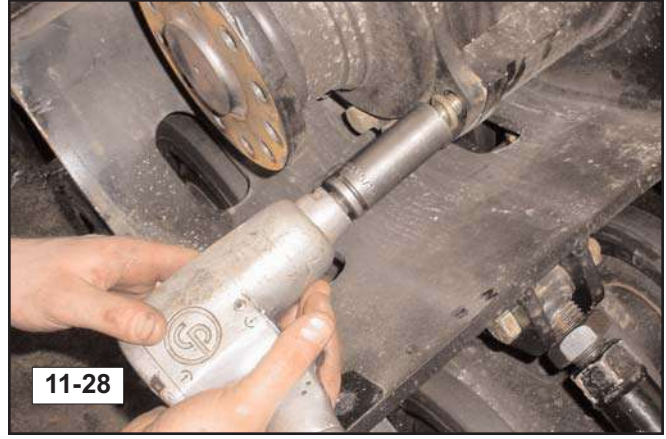
11. Remove the bolts securing the drive motor to the drive table. (fig. 11-28)
