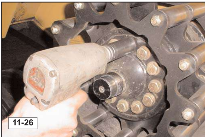
9. Remove the bolts securing the sprocket to the drive motor. (fig. 11-26)
