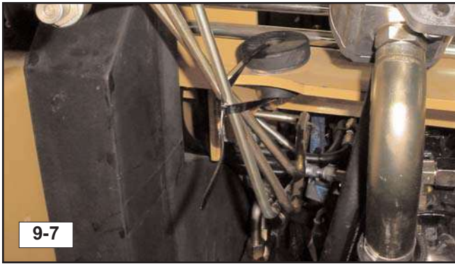
9. Gently move the hard lines out of the way to allow for reservoir removal then zip tie them to the motor mount to keep them secure. (fig. 9-7)
