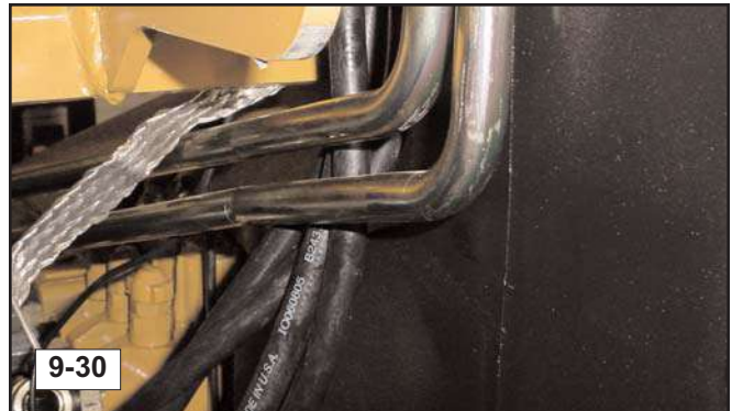
28. Slide the various control hoses to the side of the reservoir (tank) so that they do not interfere with the tank moving upwards in the chassis. (fig. 9-30)
