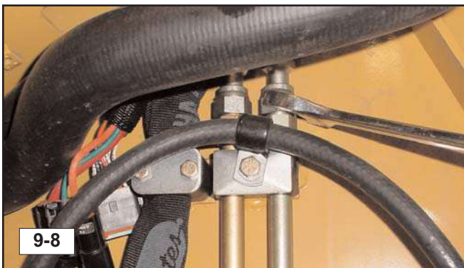
10. Disconnect the bucket cylinder hoses from the hard lines in the upper right portion of the engine compartment. Remove all line clamps. (fig. 9-8)
