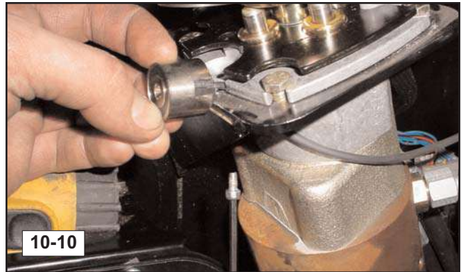
10. Remove the fittings on the back of the joystick (lift arm control joystick only). (fig. 10-7)
