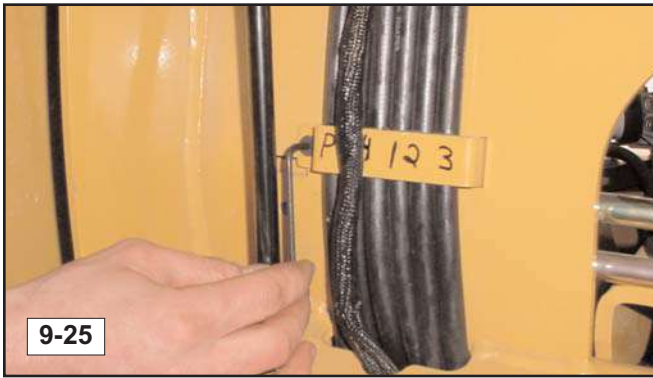
23. Remove the lower hose restraints to allow the hoses to be pulled through the chassis. (fig. 9-25)
