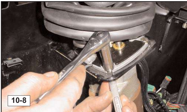
11. Remove the bolts and nuts securing the joystick to the mounting bracket. (fig. 10-8)
