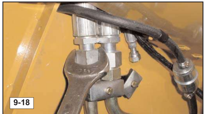
17. Disconnect the auxiliary hydraulic lines from the lift arm control valve and the hoses leading to the quick coupler lines on the lift arm. (fig. 9-17, 9-18)
