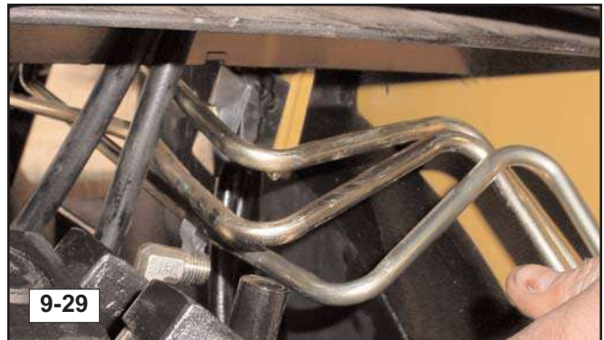
27. Slide the quick attach and test port tubes forward so that they do not interfere with the reservoir (tank) moving upwards in the chassis. (fig. 9-29)
