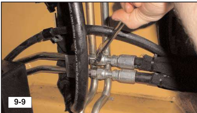
11. Disconnect the lift cylinder hoses from the hard lines to allow the bucket cylinder lines to be removed. (fig. 9-9)
