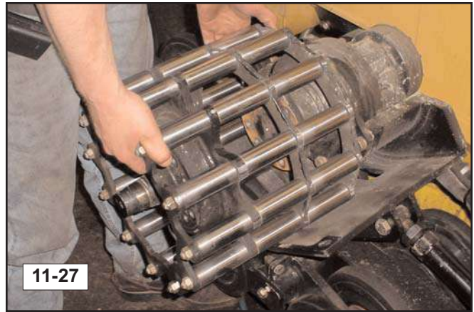
10. Remove the sprocket assembly from the undercarriage. (fig. 11-27)
