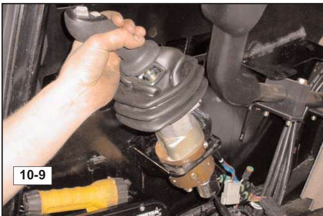
12. Lift the joystick through the opening in the bracket and remove it from the machine. (fig. 10-9)
