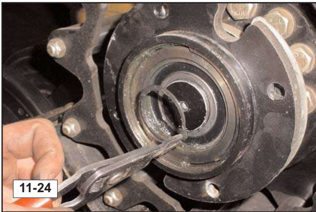
7. Remove the snap ring securing the bearing assembly to the outer sprocket shaft. (fig. 11-24)
