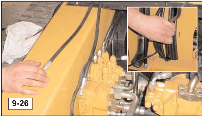
24. Pull the hoses up through the chassis opening and lay them aside as shown (both sides). (fig. 9-26)
