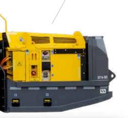
Epiroc's self-sustained battery, which has its own dedicated cooling system, allows for both on-board and off-board charging.
