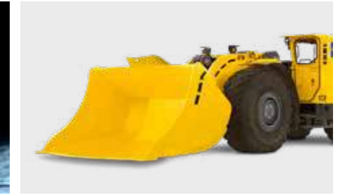
Innovative boom/bucket design and load-sensing hydraulics ensures one-pass mucking while minimizing the fuel consumption.
