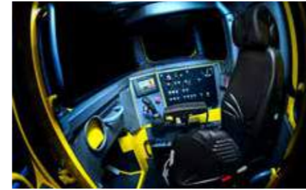
The comfortable, ROPS and FOPS certified cabin is air conditioned and features the unique Epiroc footbox to maximize leg room.
