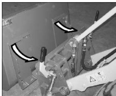
Figure 46 – Standard All-Tach® System Hitch Removal
