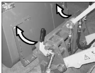
Figure 47 – Hydraulic Power-A-Tach® System Hitch Positioning
