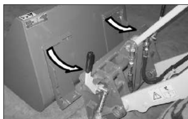
Figure 52 – Hydraulic Power-A-Tach® System Hitch Removal
