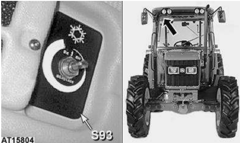
S93 - Heating and air-conditioning switch
