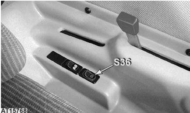
Beacon light switch
