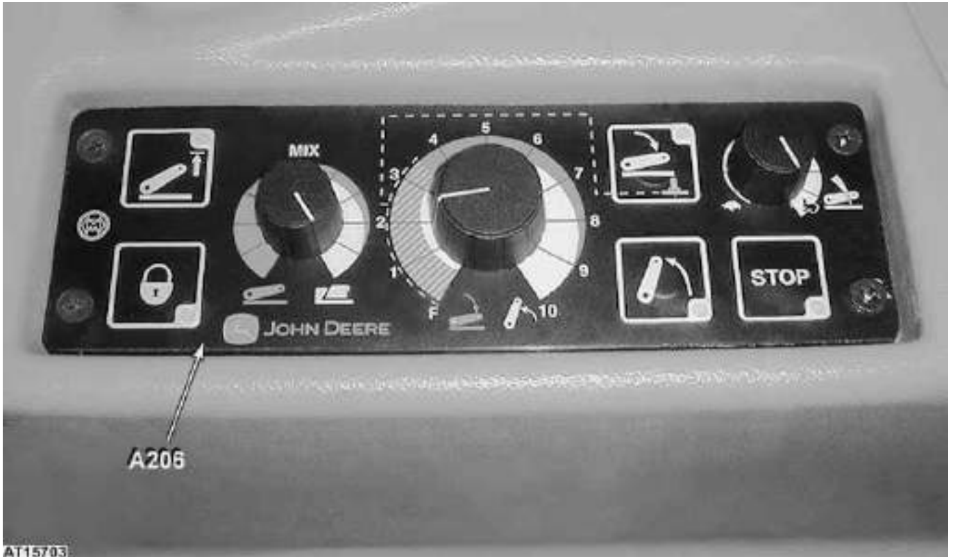
EHS control panel
