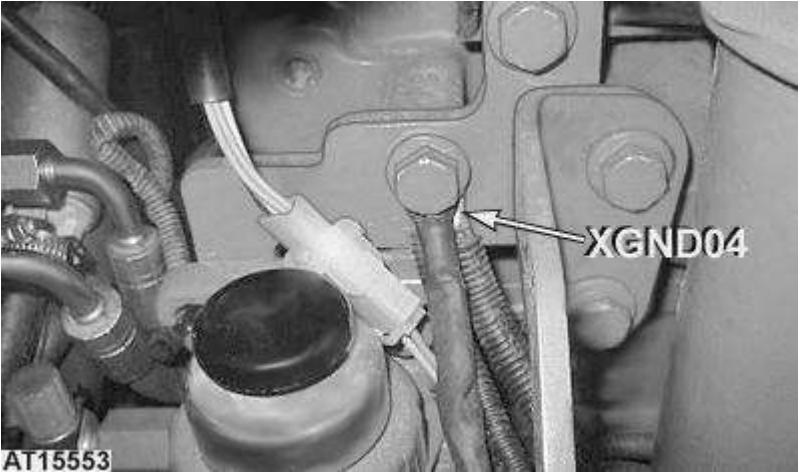
XGND04 - ground connection W10
