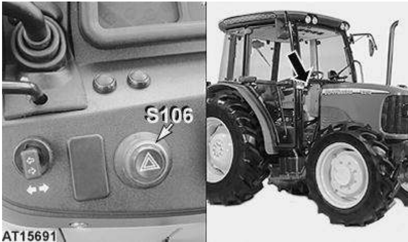
S106 - hazard warning light switch
