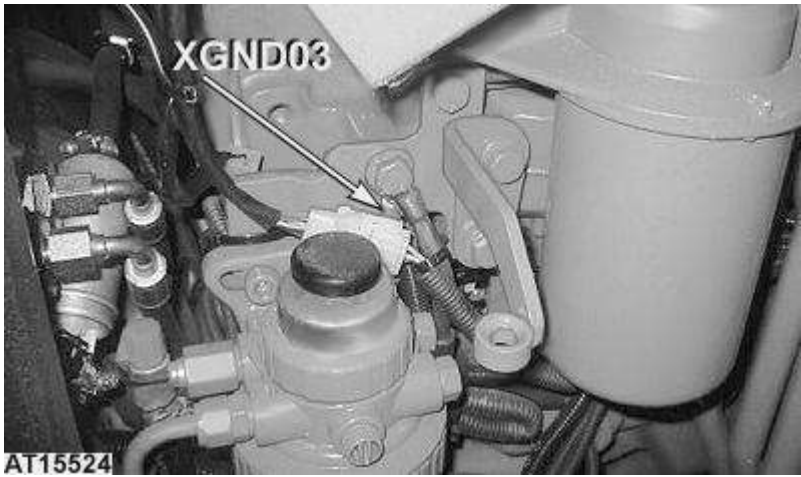
XGND03 - ground connection W04
