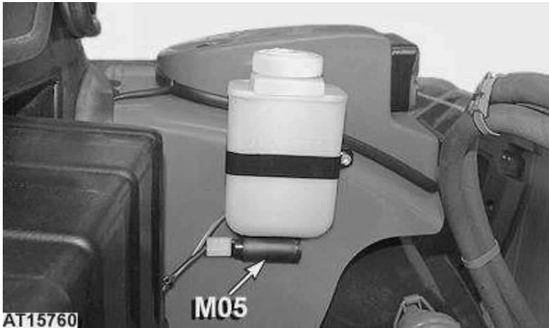
Pump of washer system
