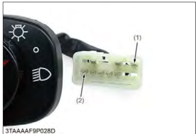
(1) Black / blue lead (A) Hazard switch ON position (2) Blue / white lead
