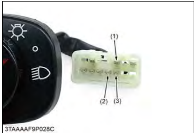
(1) Green lead (2) Red / white lead (3) Green / white lead (A) Turn signal light switch LEFT position
