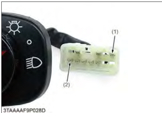
(1) Black / blue lead (A) Hazard switch OFF position (2) Blue / white lead
