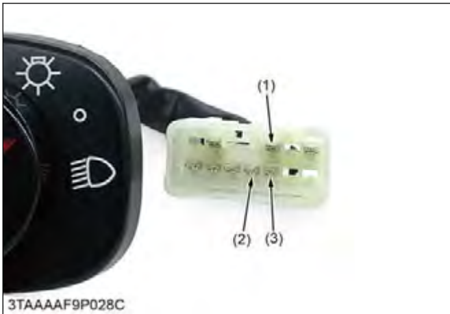
(1) Green lead (2) Red / white lead (3) Green / white lead (A) Turn signal light switch RIGHT position
