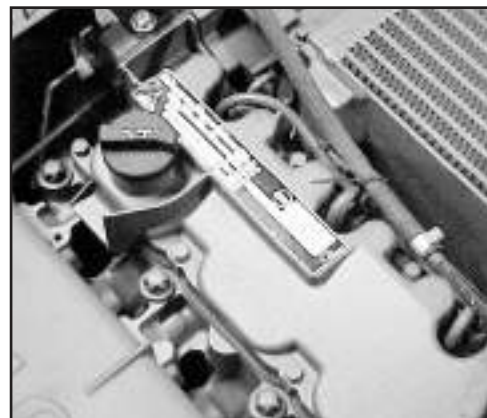
Engine identification. The manufacturer's plate C is on the valve cover.
