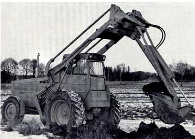
Narrow trenching for pipes or power cables, using a hydraulic excavator boom with 180° swing arc.
