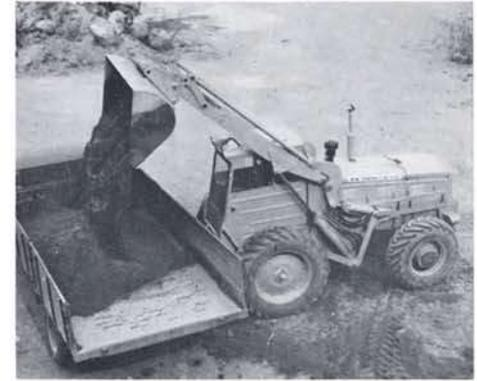
The BM-VOLVO implement attachment system permits the use of a very wide range of standard attachments. Because attachments can be changed so speedily, machines can be properly equipped for each job without unnecessary loss of time. The profitability of a loader is greatly dependent on the use of the right tool for the job and the line of
