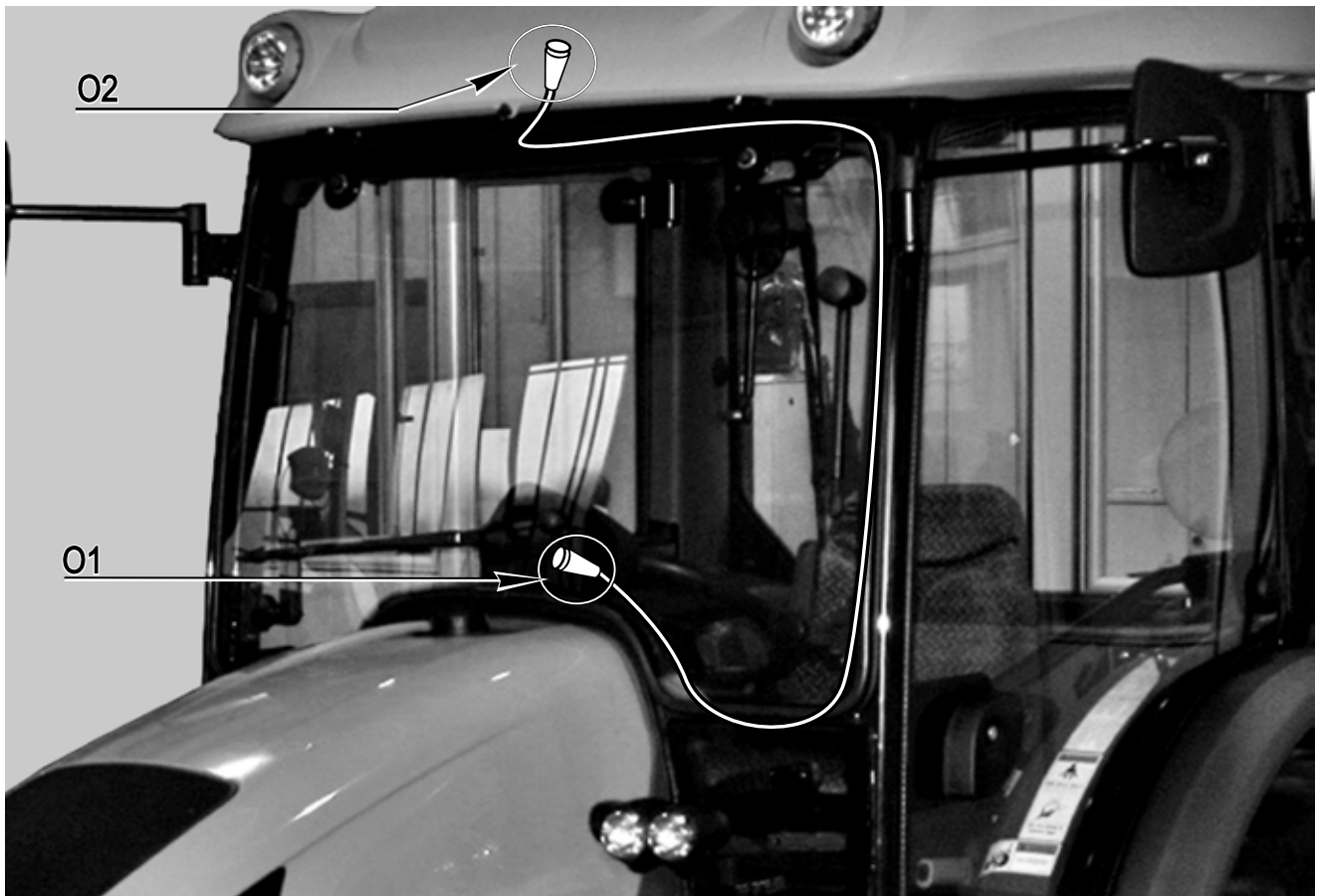
Fig. 1308 - Positions of windscreen wiper wiring connectors
