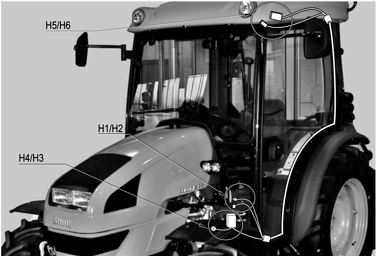
Fig. 1282 - Positions of cab power supply wiring connectors
