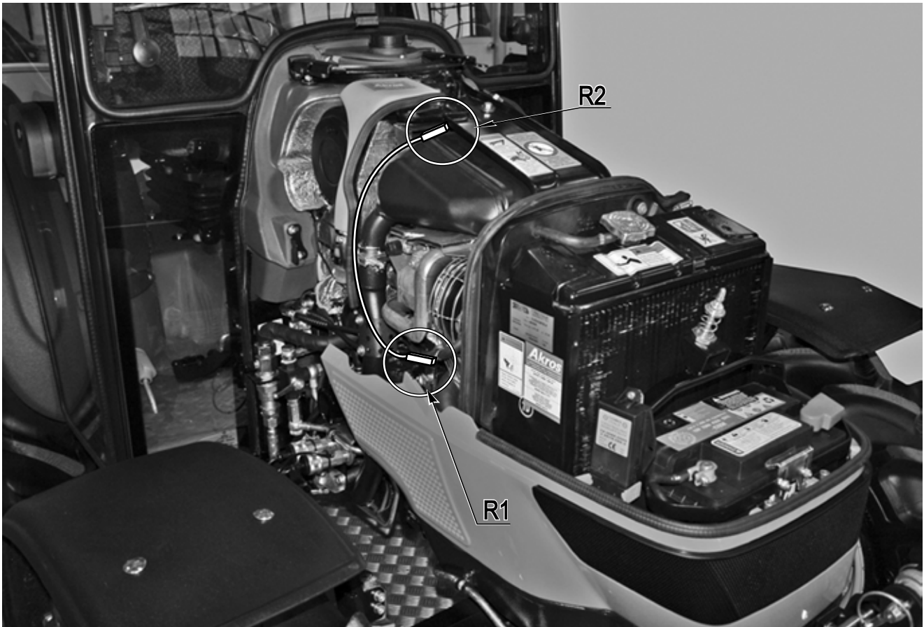
Fig. 1201 - Positions of compressor wiring connectors
