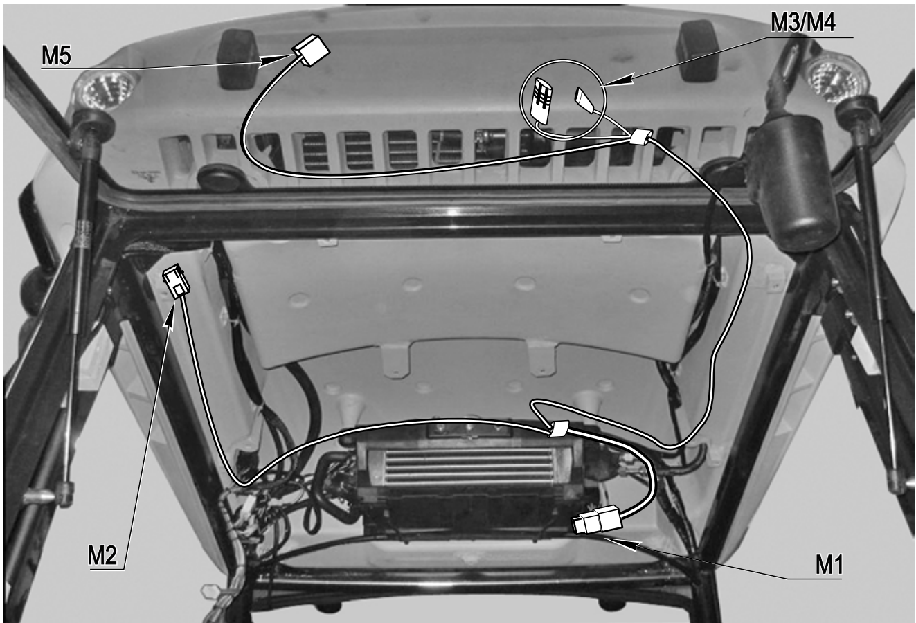
Fig. 1286 - Position of air conditioner wiring connectors
