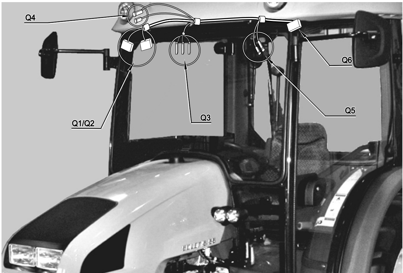
Fig. 1312 - Positions of radio-loudspeaker wiring connectors
