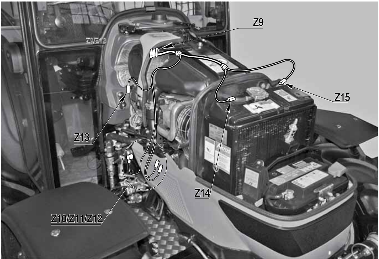
Fig. 1180 - Positions of front wiring connectors (2/2)
