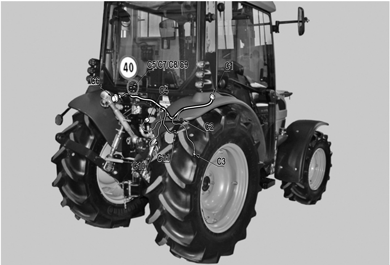
Fig. 1260 - Positions of rear wiring connectors
