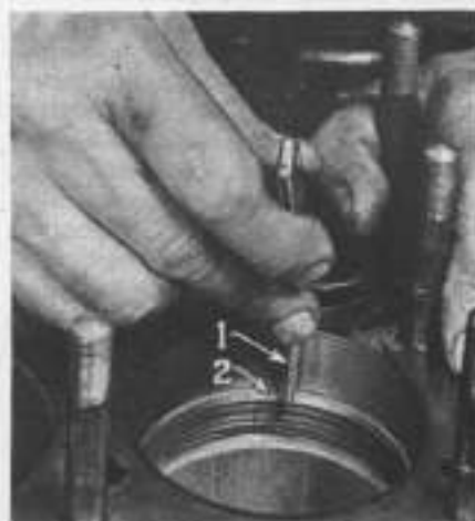
Fig. MH145—Checking ring gap.
