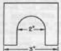
Fig. MH 337—Special washer for removing mainshaft—Models 20, 20K, 22, 22K, 81 and 82.
