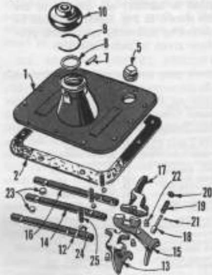
Fig. MH 330—Models 22 and 22K transmission cover and shifters. Models 20, 20K, 81 and 82 are similar.
