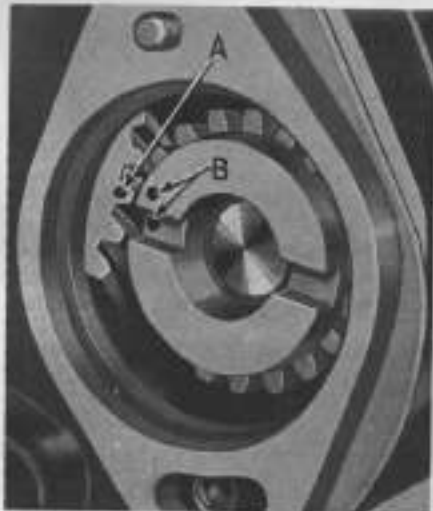
Fig. MH 242—Magneto drive timing marks on models 101 Jr., 102 Jr. and 102 G. Jr.
