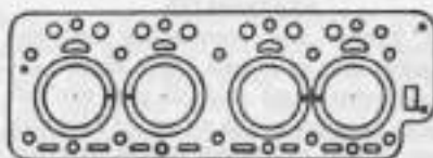
Fig. MH143—Massey-Harris cylinder sleeves are installed properly when "dots" on upper flange of sleeves are in the position shown.
