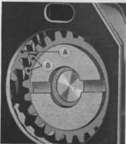
Fig. MH 243—Magneto drive timing marks on models 101 Sr., 102 Sr. and 102 G. Sr.
