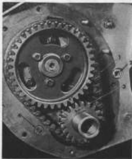
Fig. MH135—Correct arrangement of timing marks on Chrysler engine. On T57 engines, screw (4) must be removed before front main bearing cap can be removed.
