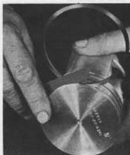
Fig. MH144—Checking piston ring side clearance.
