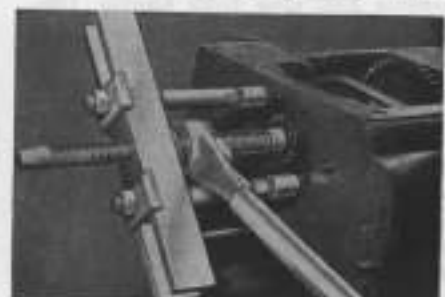
Fig. MH 312—Pressing out belt pulley and P.T.O. drive gear shaft using OTC tool no. 938.
