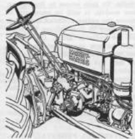
Fig. MH105—Massey-Harris model 55 steering gear installation.
