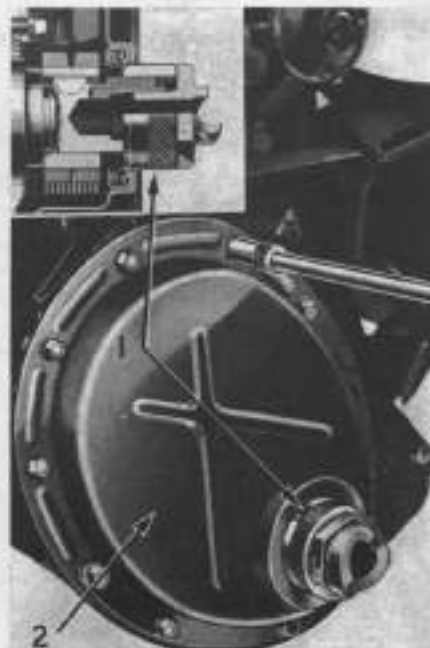
Fig. MH140—Crankshaft front oil seal aligning tool being used on Chrysler engine.
