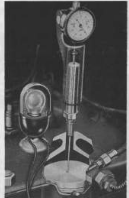
Fig. MH 241—Special timing tool installed for checking ignition timing on Massey-Harris tractors equipped with Chrysler engines.
