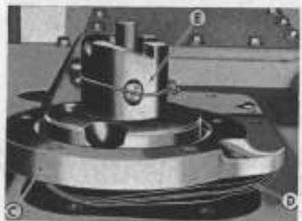
Fig. MH450—Power lift adapter and drive clutch—models 20, 20K, 81 and 82—Showing adapter plate "C", shims "D" and clutch jaw "E".
