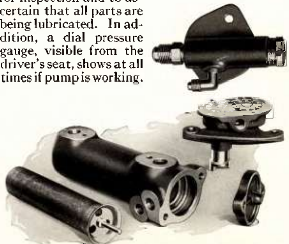
Showing Force Feed Oil Pump—Oil Sump, Oil Filter Screen and Pressure Adjustment.
