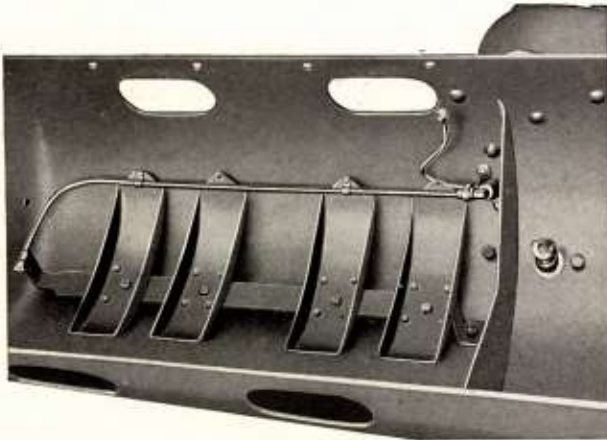
Showing Oil Dip Pans in U Frame with Oil Delivery Pipe Fastened to Pans—Also Flexible Pump Connection Inside of Frame. A Hole in the Curved End of Oil Pipe Throws a Constant Stream of Oil to the Timing Gears.
