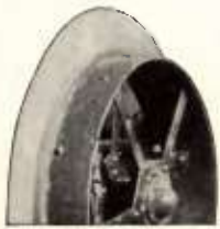
Showing skid band attached to front wheel as used when cultivating with the Wallis "Certified" Tractor Guide.
