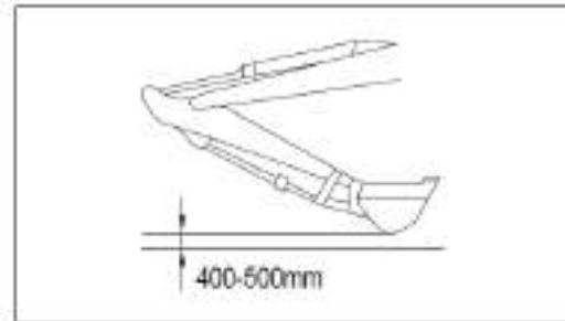
Figure 4-25 The position of the working device while the machine is moving forward
