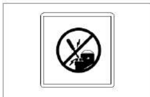
Figure 1-22 Prohibit from hot-wiring the machine
