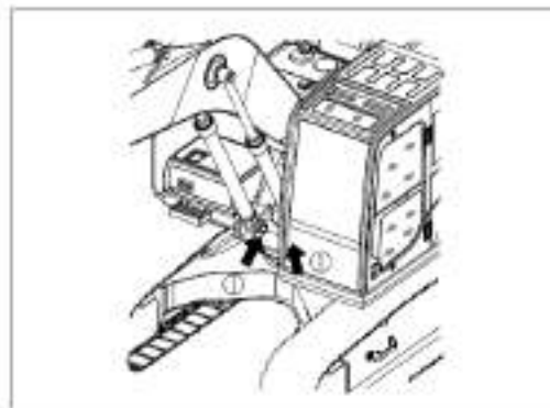
Figure 4-2 Lubricate the work device ( I )
