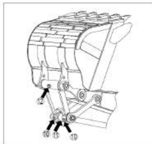
Figure 4-6 Lubricate the work device (V)
