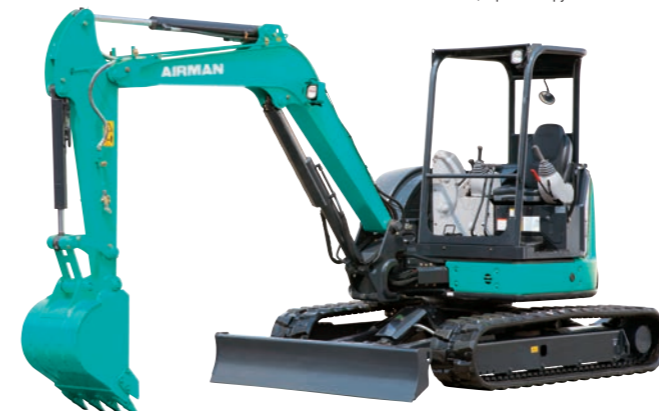
AX48u-7 Operating weight 4,770kg Capacity 0.11m 3 Rubber shoes, 4-pole canopy
