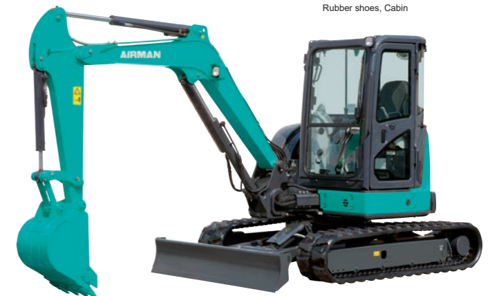
AX55u-7 Operating weight 5,210kg Capacity 0.14m 3 Rubber shoes, Cabin
