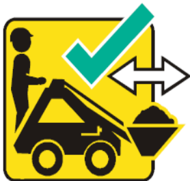
5. TRANSPORT MATERIAL WITH BUCKET DOWN AND LEVEL
