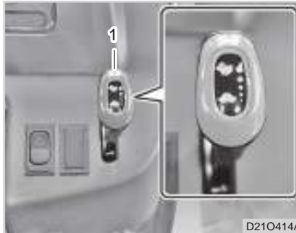
(1) Hand Throttle Lever 🐢 : Slow 🐰 : Fast
