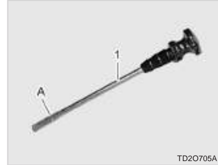
(1) Oil Dipstick (A) Upper Limit
