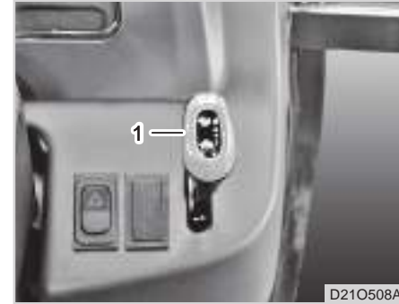
(1) Hand Throttle Lever 🐢 : Slow ➡ : Fast
