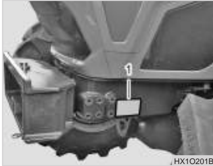
(1) Tractor Serial Number Plate
