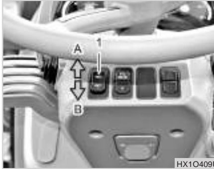
(1) PTO Restart (Res +)/Setting (Set -) Switch (A) Restart (Res +) (B) Setting (Set -)
