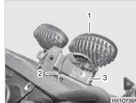
(1) LED work lamp (2) Wiring (3) Work lamp mounting bracket
