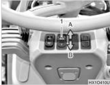
(1) PTO Cruise ON/OFF Switch (A) ON (B) OFF
