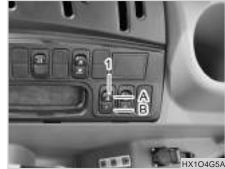
(1) Driving Selection Switch (A) 4WD (B) OFF
