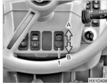
(1) Hazard Lamp Switch (A) ON (B) OFF
