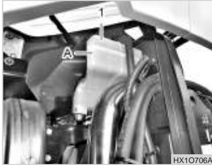
(1) Reservoir Tank (A) Min (Lack)
