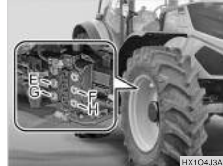
(E) Bucket Roll Back (F) Bucket Dump (G) Boom Down (H) Boom Up
