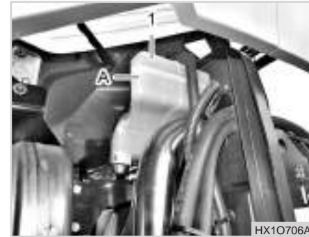
(1) Reservoir Tank (A) MIN (Lack)
