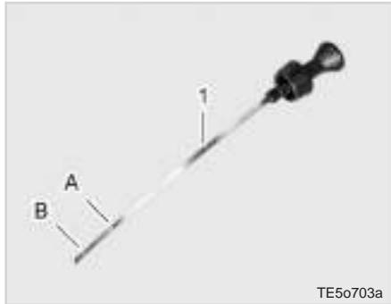
(1) oil Dipstick (a) upper limit
