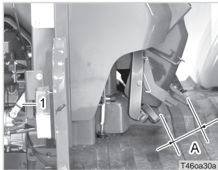
(1) Clutch rod (a) free Travel
