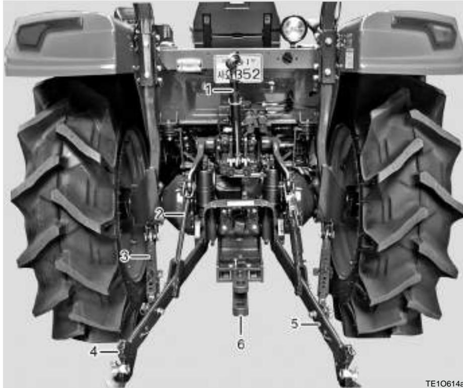
(1) Top Link (2) Crank Lifting Rod (3) Lifting Rod (4) Telescopic Stabilizers (5) Lower Link (6) Draft hitch
