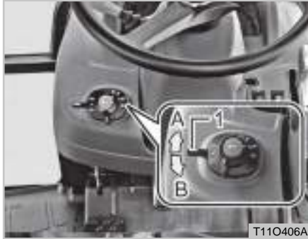
(1) Turn Signal Light Switch (A) Right Turn (B) Left Turn
