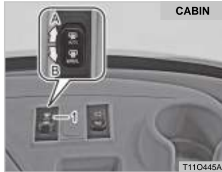
(1) PTO Selection Switch (A) AUTO (B) MANUAL
