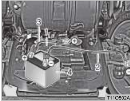
(1) Dead Battery (2) Jumper Cables (-) (3) Jumper Cables (+) (4) Helper Battery
