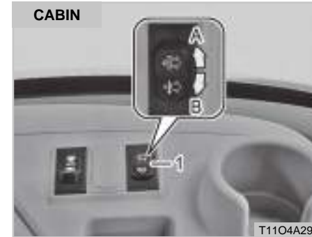
(1) Regeneration Underway Lamp (A) Activation (B) Deactivation
