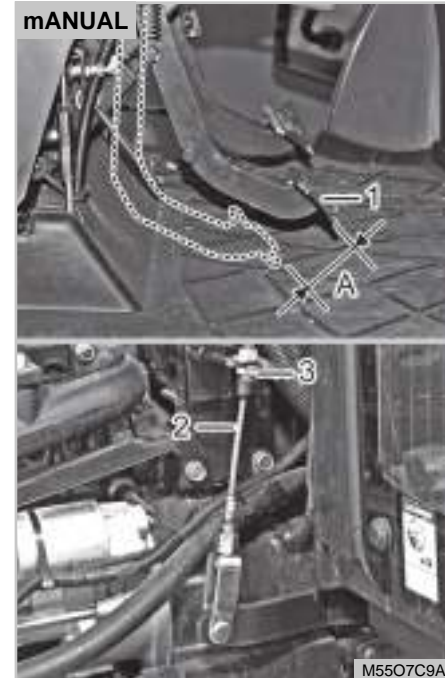
(1) Clutch Pedal (2) Clutch Cable (3) Lock Nut (A) Free Play
