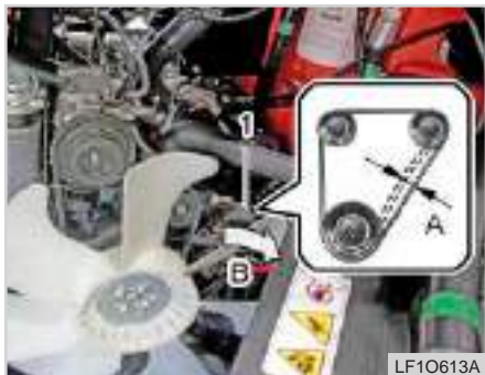
(1) Adjusting Bolt (A) Adjusting Belt Tension (B) Pull
