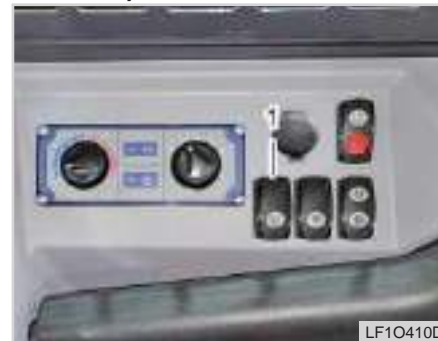
(1) Beacon lamp switch
