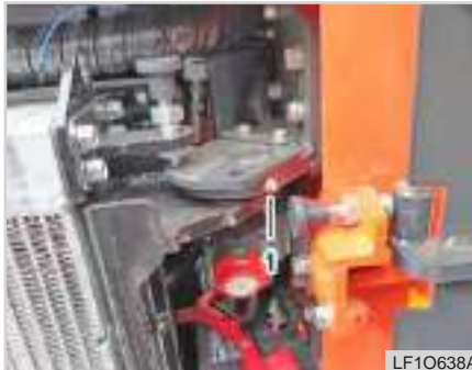
(1) Upper part of the opening of the engine compartment
