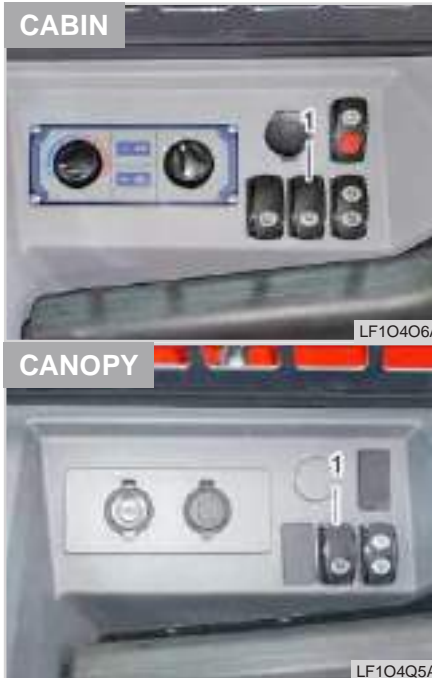
(1) Interior lamp ON/OFF switch
