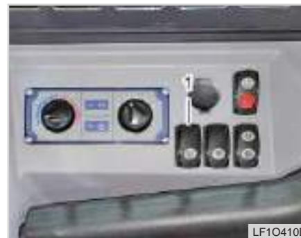
(1) Beacon lamp switch
