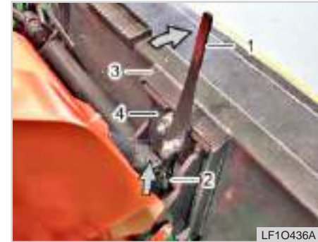
(1) Hand lever (2) Locking pin (3) Bucket slot (4) Implement holder
