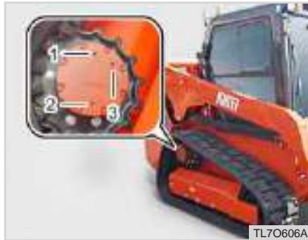
(1) Filler hole (2) Drain plug (3) Oil check hole
