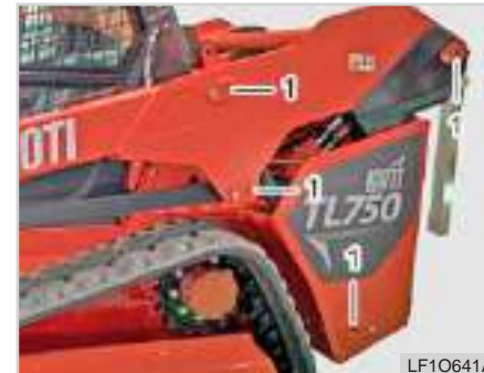
(1) upper/lower parts of the lift arm cylinder
