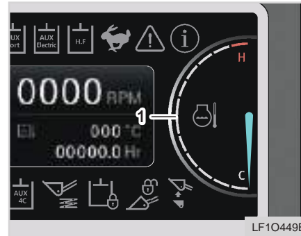
(1) Engine coolant temp. gauge
