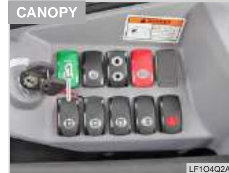
(1) AUX (Auxiliary Hydraulics) port switch
