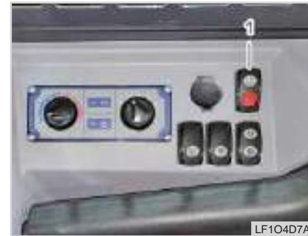
(1) Hydraulic quick attach switch
