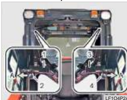
(1) Door Stopper, RH (2) Handle (Lock Pin), RH (3) Door Stopper, LH (4) Handle (Lock Pin), LH (A) Lock
