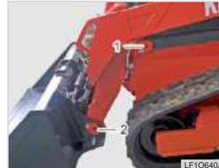
(1) Lift arm cylinder (2) Hing pin area
