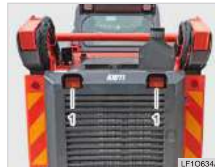
1) Brake lamp and turn signal lamp
