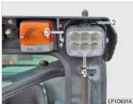
(1) LED work lamp (2) Wiring (3) Work lamp mounting bracket
