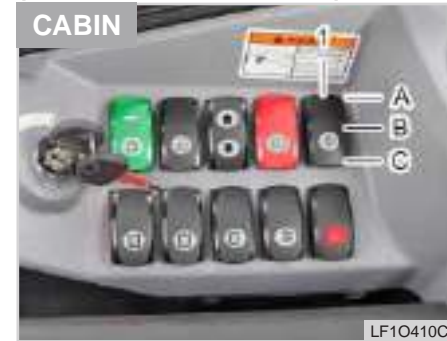
(1) Wiper / washer switch (A) OFF (B) Step 1 (C) Step 2
