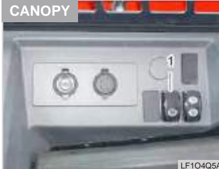
(1) Interior lamp ON/OFF switch
