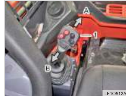
(1) Left joystick control lever (A) Forward (B) Reverse
