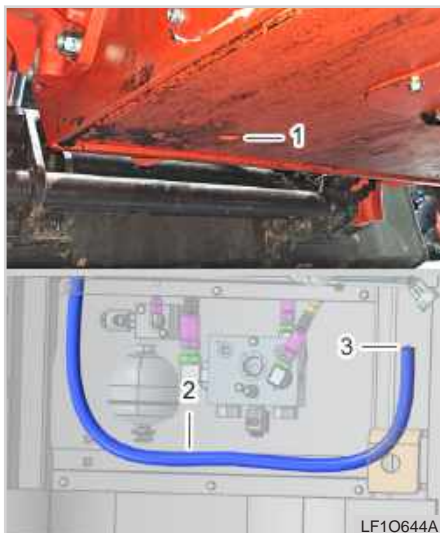
(1) Drain hole (2) Drain hose (3) Plug
