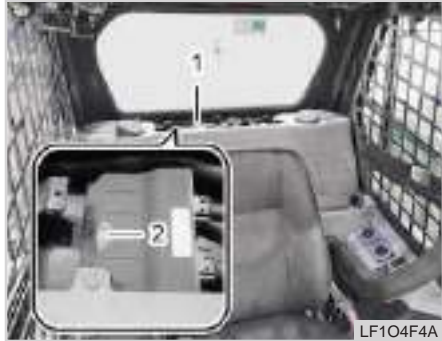
(1) MCU (Machine Control Unit) (2) Lamp
