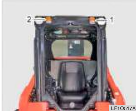
(1) Turn signal lamp (LH) (2) Turn signal lamp (RH)
