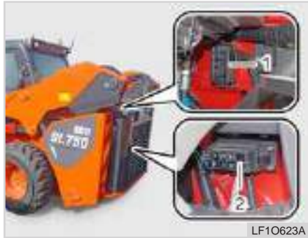
(1) Body fuse box (2) Body relay box
