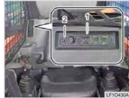
(1) Radio speakers with bluetooth (2) Power (PWR) switch
