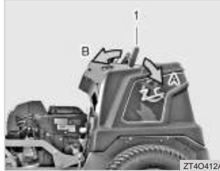
(1) Parking Brake Lever (A) Engaged (B) Disengaged
