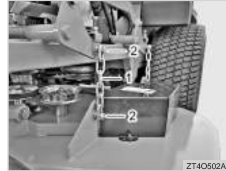
(1) Lift Link (2) Mounting Hardware
