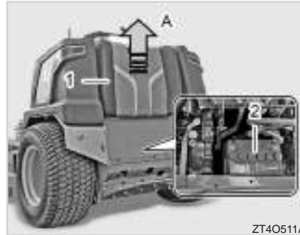
(1) Rider Platform Cushion Pad (2) Battery (A) Pull Up
