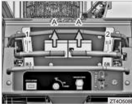
(1) LH Steering Levers (2) RH Steering Levers (A) Forward
