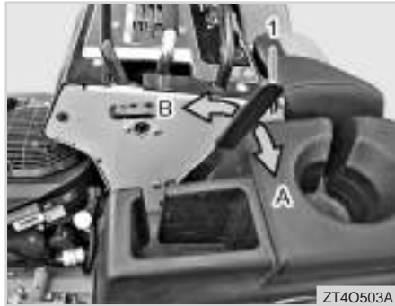
(1) Parking Brake Lever (A) Engage (B) Disengage
