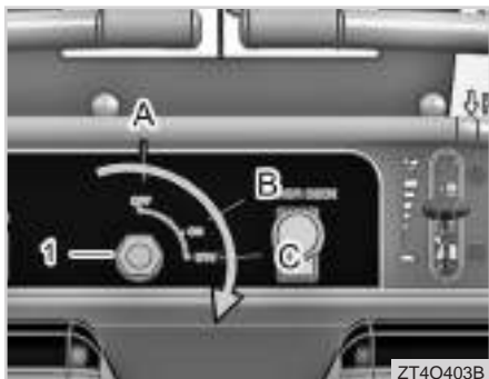
(1) Key Switch (A) OFF (B) ON (C) START
