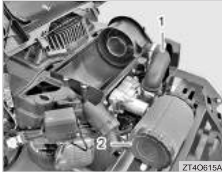
(1) Suction Hose (2) Air Cleaner Element
