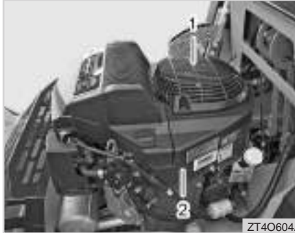
(1) Air Intake Screen (2) Engine Shroud
