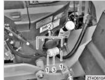
(1) Pipe Clamp (2) Fuel Line (3) Fuel Filter
