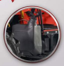
Fuel tank with a capacity of **55 liters** that provides uninterrupted operation throughout the day.
