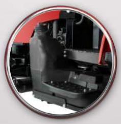
Fuel tank with a capacity of **60 liters** that provides uninterrupted operation throughout the day.
