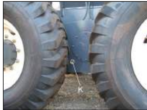
Fig. 274 Check oil level of tandem axle BG 110
