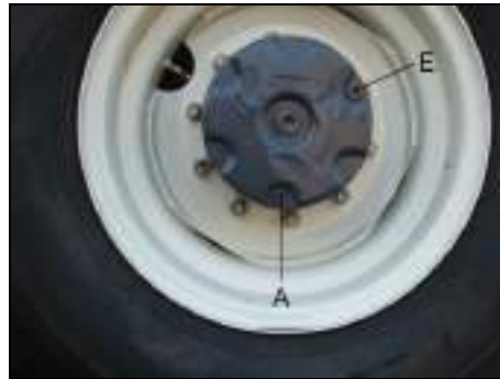
Fig. 293 Oil change wheel hubs oil drain openings A and E BG 130 / BG 160
