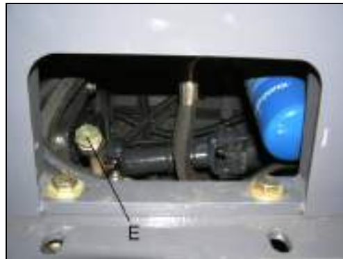
Fig. 300 Oil change axle gear fill screw - BG 190
