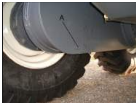
Fig. 305 Tandem oil change - oil drain screws - BG 190
