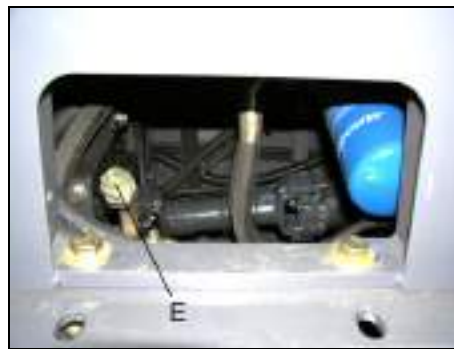
Fig. 289 Oil change axle gear BG 130 / BG 160
