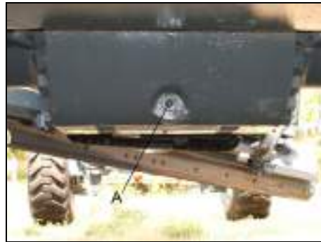
Fig. 288 Oil change rear axle BG 130 / BG 160
