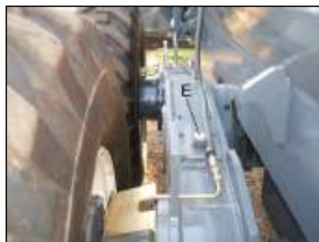
Fig. 291 Tandem oil change oil fill opening BG 130 / BG 160
