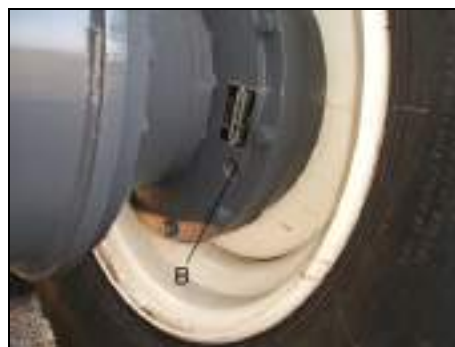
Fig. 294 Oil change wheel hubs drain opening B BG 130 / BG 160
