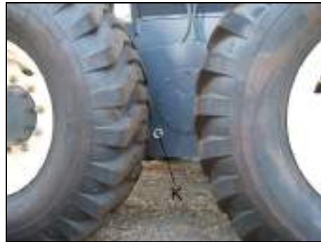
Fig. 290 Tandem oil change - check window BG 130 / BG 160
