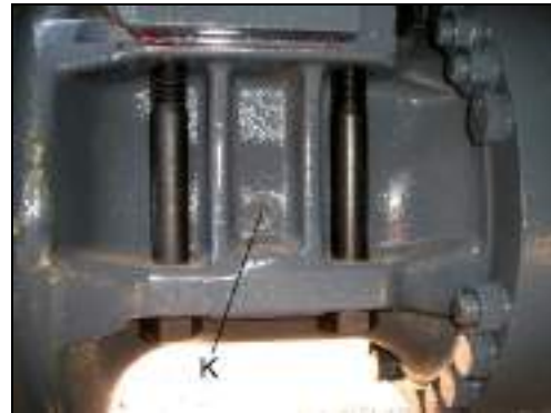
Fig. 296 Check oil level in the axle gear - BG 190
