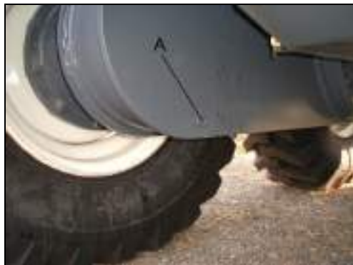
Fig. 279 Tandem oil change - drain opening
