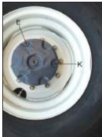
Fig. 295 Oil change wheel hubs fill screw E and check screw K BG 130 / BG 160
