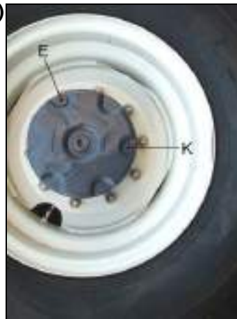
Fig. 287 Check oil level in wheel hubs BG 130 / BG 160
