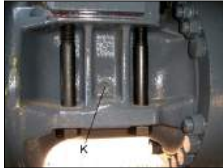
Fig. 285 Check oil level in the axle gear BG 130 / BG 160
