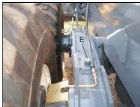
Fig. 304 Tandem oil change - fill opening - BG 190
