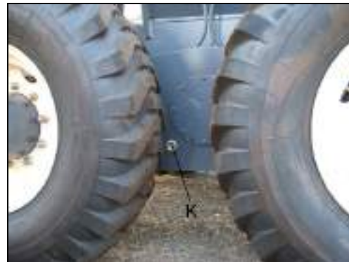
Fig. 297 Check oil level in the tandem - check screw BG 190
