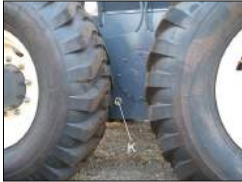
Fig. 277 Tandem oil change - check window
