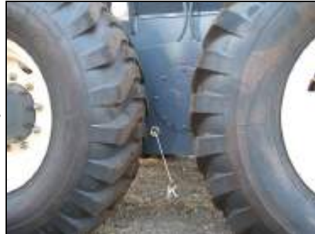
Fig. 303 Tandem oil change oil - check screw - BG 190
