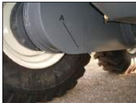
Fig. 292 Tandem oil change oil drain screws BG 130 / BG 160
