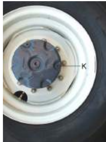
Fig. 275 Check oil level in wheel hubs
