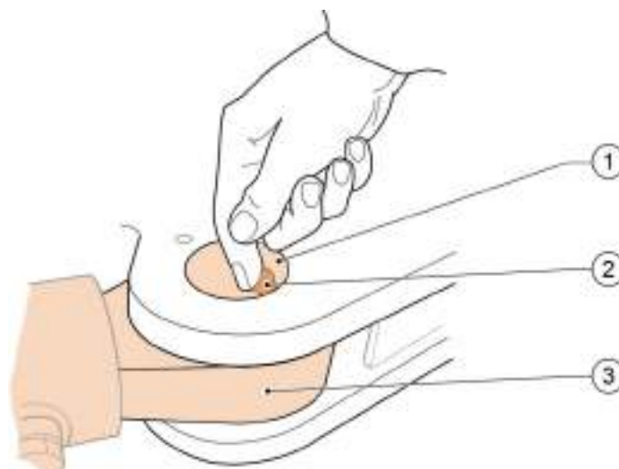
Fig. 203 Lubricate cylinder base bearing
