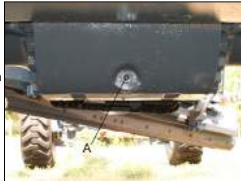
Fig. 299 Oil change axle gear drain screw - BG 190
