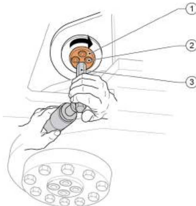
Fig. 176 Tighten all screws on the cover below
