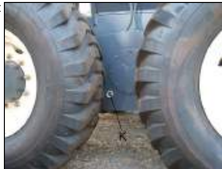
Fig. 286 Check oil level in the tandem BG 130 / BG 160
