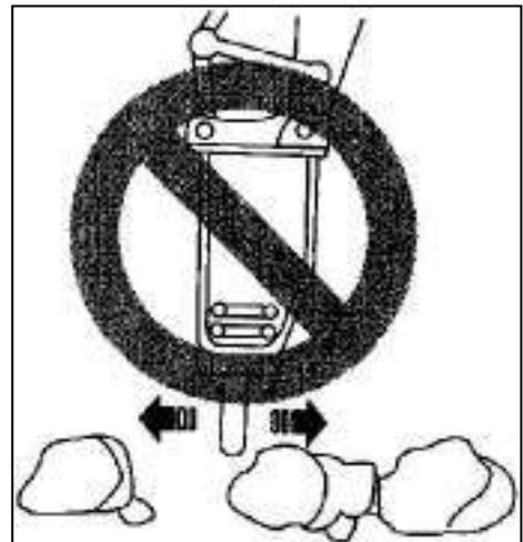
Do not swivel the hydraulic hammer when working on rocks, concrete and so on.
