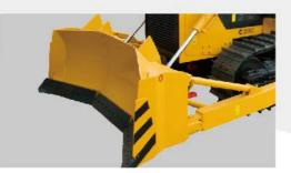
Equipped with straight-tilting shovel as standard as well as U shovel and angle shovel as options, all provided with well durable blade
