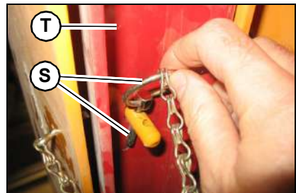
Figure 11 – Lift Arm Support Storage Lynchpin Removal
