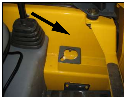
Figure 1 – Fire Extinguisher Location
