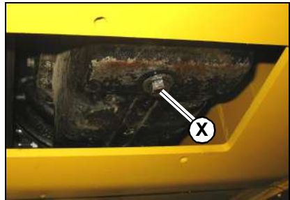
Figure 95 – Engine Oil Drain Plug
