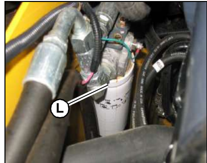
Figure 110 – Hydraulic Oil Filter
