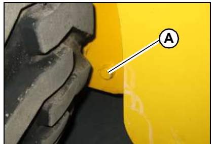
Figure 96 – Model 1650R Remote Engine Oil Drain Plug Location
