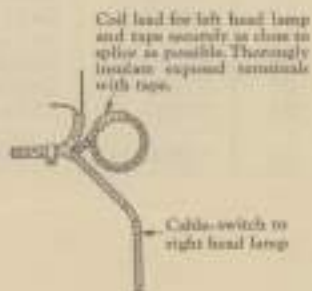
Illustration No. 13B Detail showing coiled left head lamp cable when right head lamp only is used.
