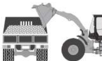
"Tip-off To Truck" Mode
