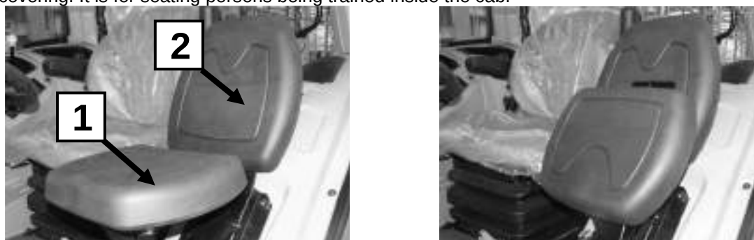
Figure 4-19 Additional seat. 1 –seat part raised upwards; 2 – seat support.
