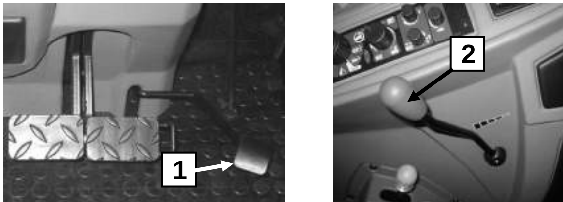
Figure 4-15a Control of engine RPM speed of PRONAR 6170 tractor . 1 – accelerator pedal; 2 – accelerator lever;
