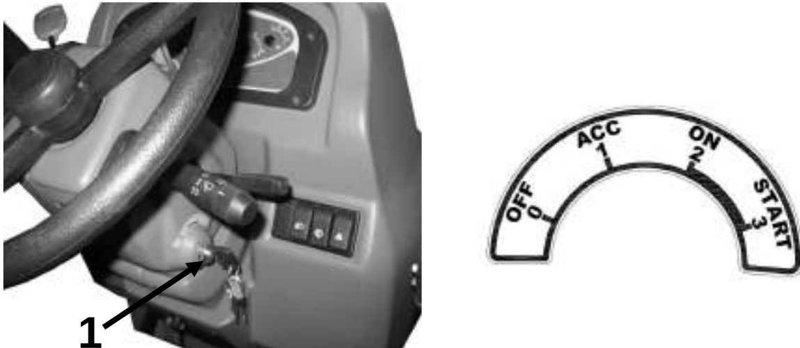
Figure 4-14 Engine start-up control. 1 – starter switch;
