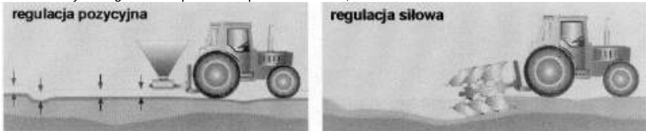
Figure 5-18 Means of adjustment applied in agricultural tractor hydraulic lifts.
