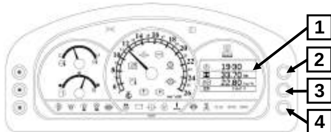
Figure 4-12b LCD of PRONAR 6180 tractors 1 - LCD display, 2 - button to change the displayed parameters, 3 - clock settings button, 4 - button to change the display colour.
