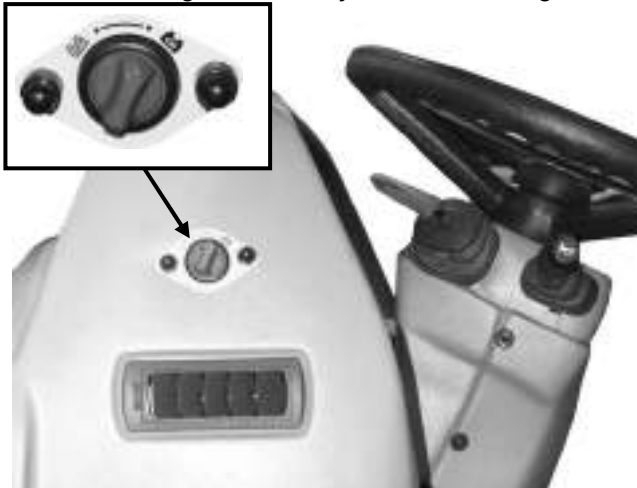
Figure 5-1 Battery switch in tractor cab.
