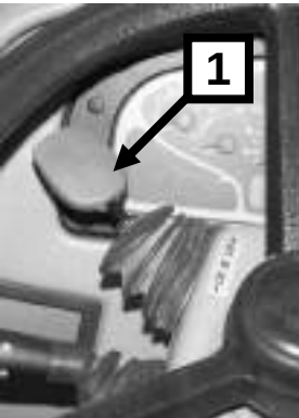
Figure 5-6. Travel direction switch and gear lever of PRONAR 8140 tractors.
