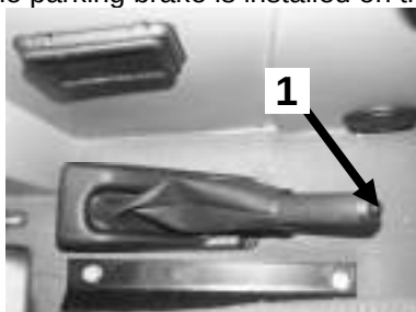
Figure 4-25 Parking brake. 1- locking button
