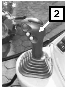
Figure 5-6. Travel direction switch and gear lever of PRONAR 8140 tractors.
