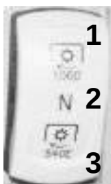
Figure 4-28 Switch connecting appropriate PTO rotation speed: 540 or 1000 revs/min.
