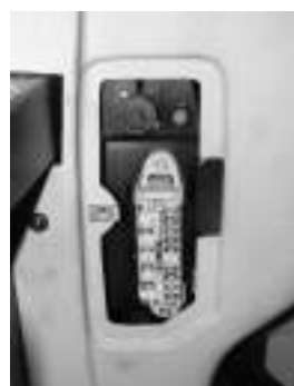
Figure 5-33 Location of set of fuses on left side of steering column. A- screw; B- cover
