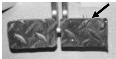
Figure 4-24 Catch locking working brake pedals.
