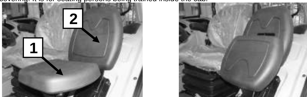
Figure 4-20 Additional seat. 1 –seat part raised upwards; 2 – seat support.
