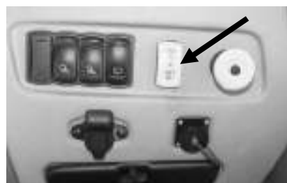
Figure 4-28 Switch connecting appropriate PTO rotation speed: 540 or 1000 revs/min.
