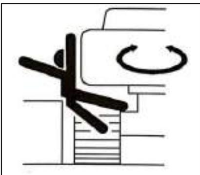
1. Before driving, place the machine to keep the bulldozers in front of the driver's seat. If the bulldozing is behind the cab, move the machine in the opposite direction (walk back and forth, turn left and right). Pay special attention when operating the machine in this case.
